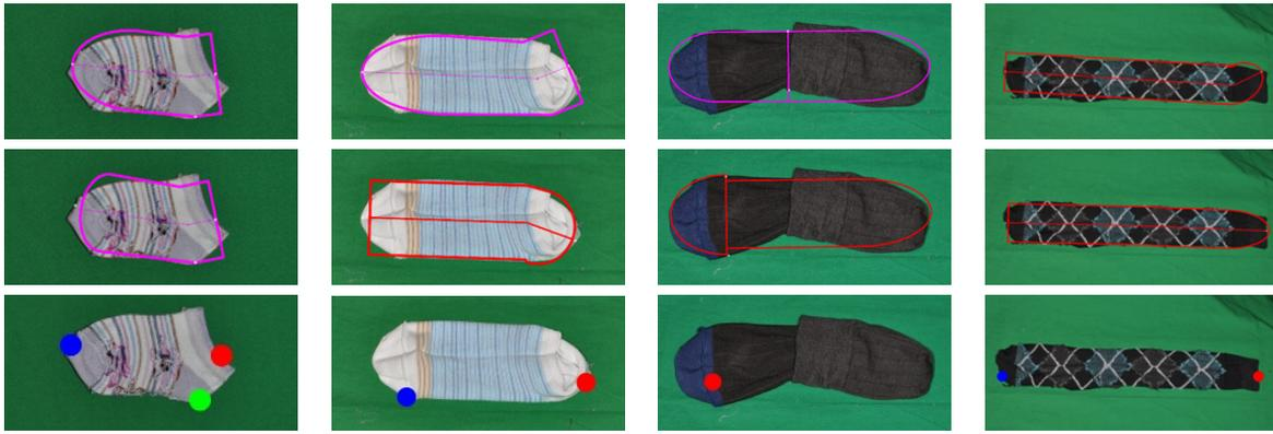
Fig. 9. Example successes and failures of the global (top), contour (middle), and appearance (bottom) models. For the appearance models, the colored circles represented the predicted landmark locations: red indicates the opening location, blue indicates the toe location, and green indicates the heel location.
